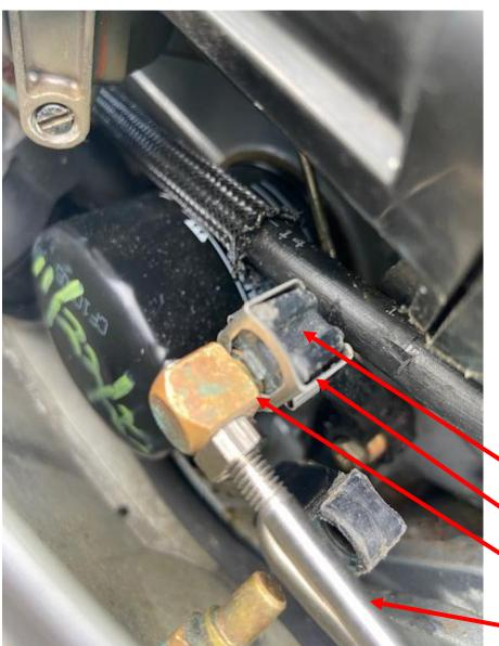
Issue is clips are not holding pivots to the linkage/levers on both the throttle and shifter. Exacerbated by the fact that they seem to bump against each other at certain activation points and the plastic levers appear worn
